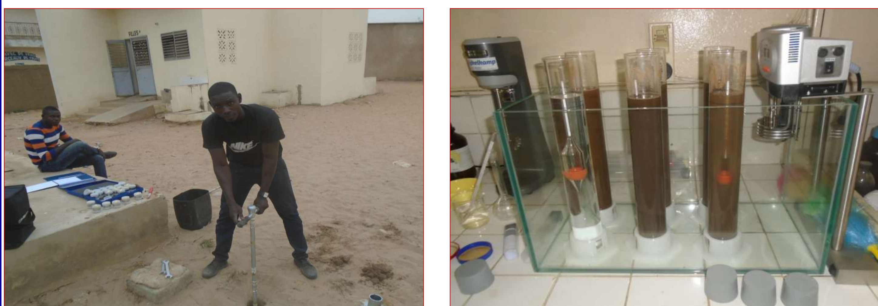
Figure 2. Field investigation (a) core sampling and lab measurements (b) hydrometer test
